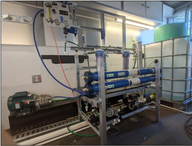
Figure 14.—Initial 2-stage membrane configuration with 20-micron and 0.2-micron prefiltration.
