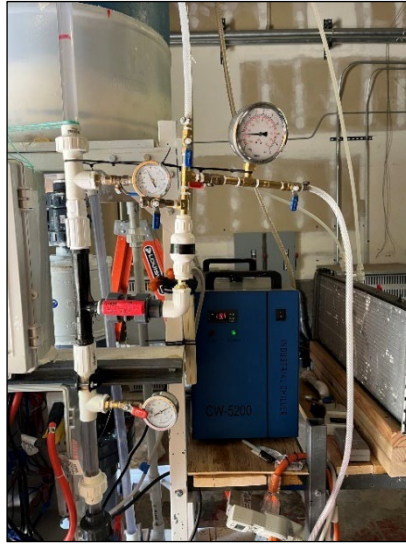
Operating variables for picture to the left: 25-psi up | 5-psi down with 21-inch Hg vacuum | chiller at 66.4°F
